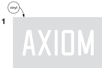
stick vinyl stencil on surface and remove masking tape
